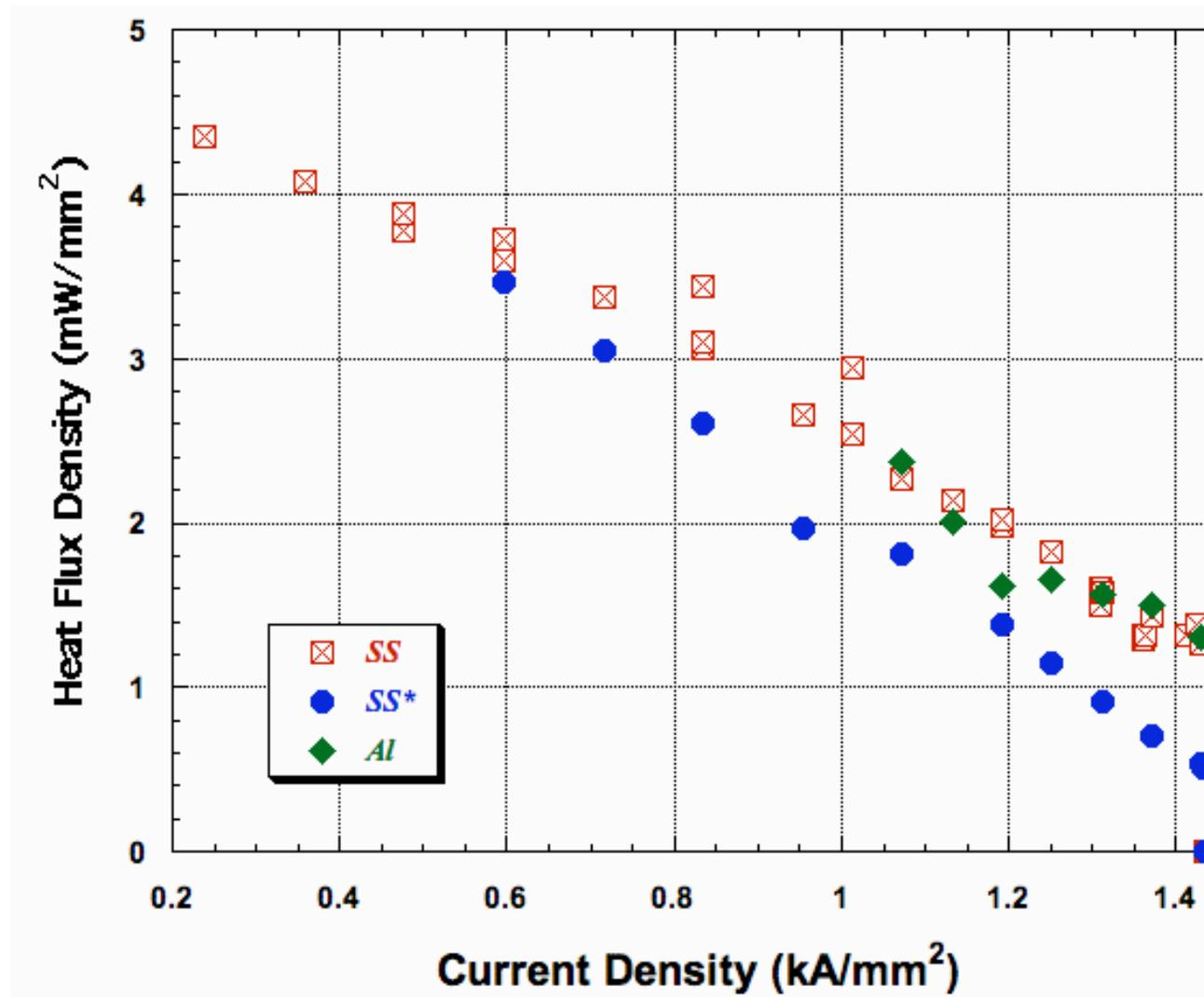
SS\* is the case with grease between mandrel and chamber so LHe is excluded
