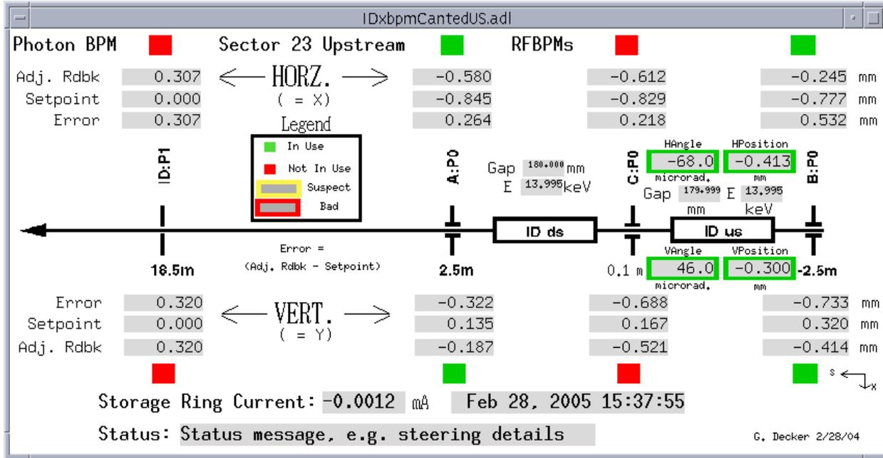
Figure 6. Full size steering display for upstream canted undulator at 23ID
