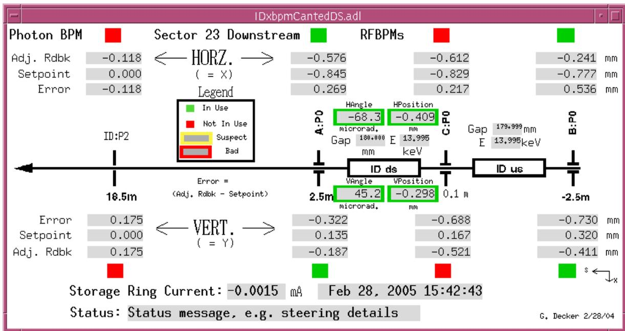
Figure 8. Full size steering display for downstream canted undulator at 23ID
