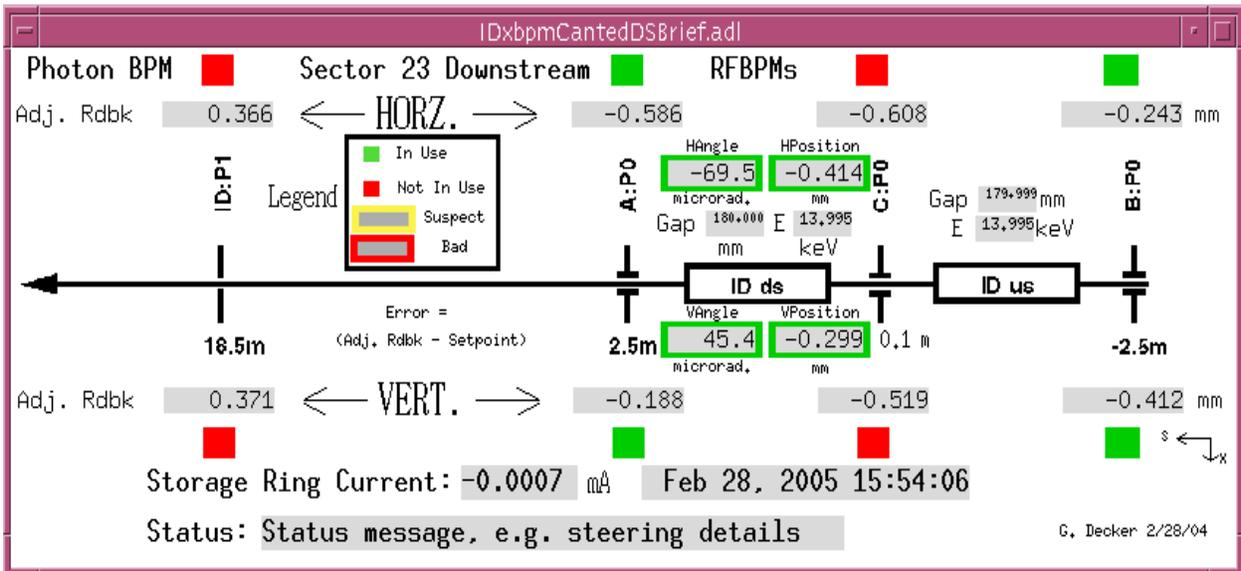
Figure 9. "Small" canted undulator display for downstream device.
