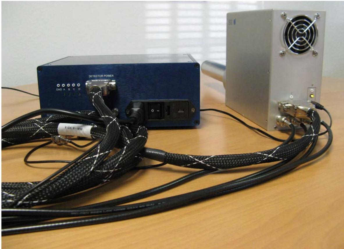
*Figure 9. Vortex-ME4™ SDD package and PS electronics box.*
