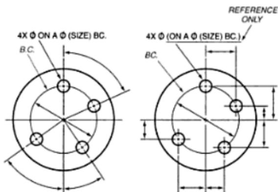
**FIGURE 10-92** Dimensioning holes around a center
