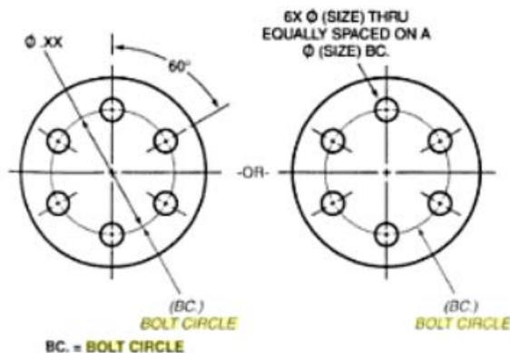
**FIGURE 10-91** Dimensioning holes on a **bolt** center diameter
