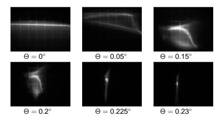
grid: 200lpi Ni mesh focus: 70  $\mu$ m V by 30  $\mu$ m (H)
