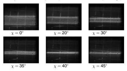
grid: 200lpi Ni mesh vert focus 35  $\mu$ m (~ 0.5 demagnified source)
