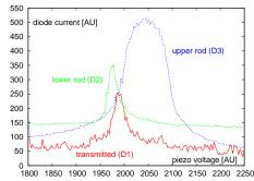
scan piezo (DAC output), acquire 3 signals on ADC inputs (D1 .. D3) find peak in transm. signal, rod signals at peak (d2, d3 to normalize stabilize on D3/d3-D2/d2
