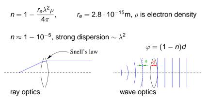
weak refraction  $\rightarrow$  many (*N*) lenses (compound refractive lens) vary f through choice of *N*
