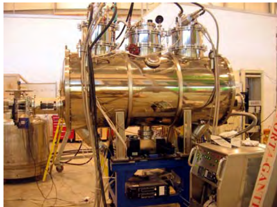
49 pole SC wiggler for Diamond Light Source by Budker Institute
