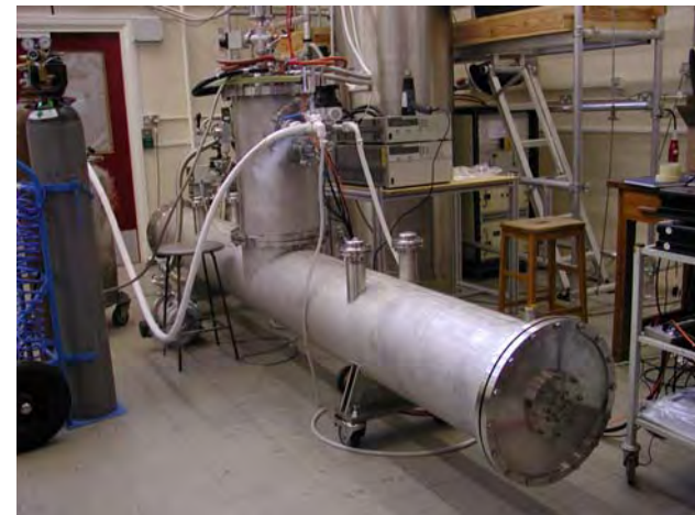
4-m long SC helical undulator built by RAL for ILC positron source project
