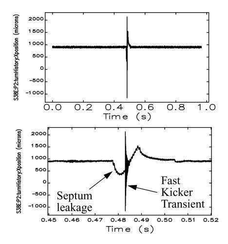
262144 turns (1 second) of data using first production model of fpga-based monopulse rf bpm data acquisition
