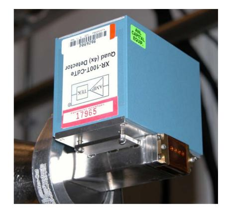
AMPTEK CdZnTe (modified from 1 element standard detector) dark current: 3 cts/hour Efficiency: 1.0 (up to 60 keV) Max. count rate: 10 kHz
