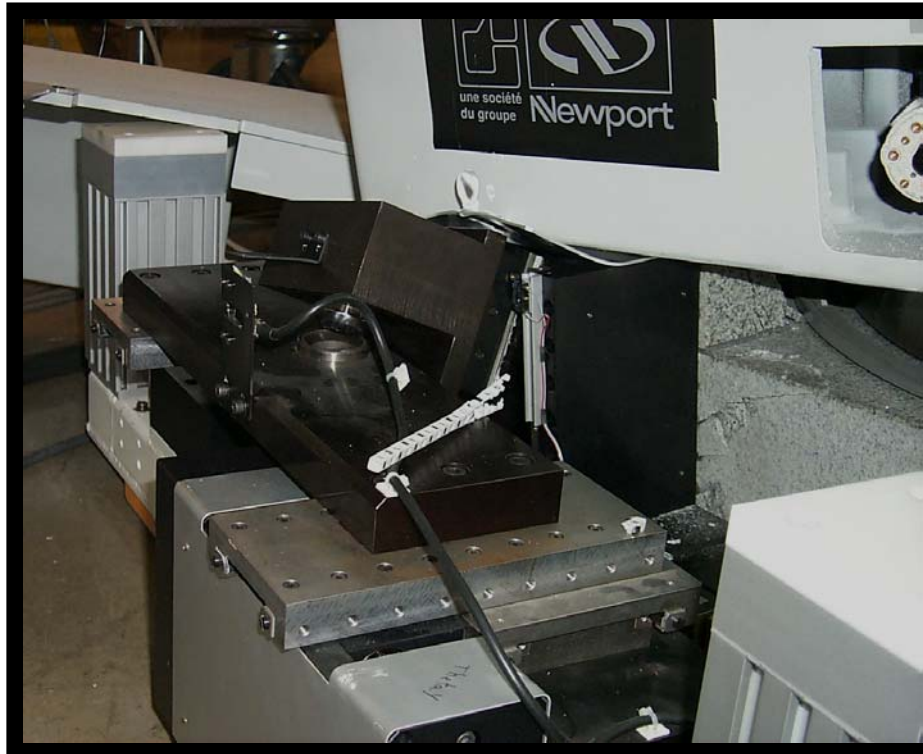
Y1 jack severely damaged, granite base cracked
