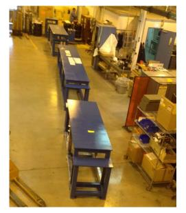
Sector mock-up to evaluate design feasibility, inform improvements needed for mechanical stability, and develop procedures. Bench measurements to back up simulations of impedance and rf behavior.
