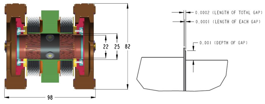
Impedance / rf heating of integrated BPM/bellows assembly (See <u>B. Stillwell</u> <u>et al., Conceptual Design and Analysis</u> <u>of a Storage Ring Vacuum Beam</u> <u>Position Monitor..., Proc. IPAC'15.</u>) Impedance / rf heating of flange gaps
