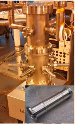
Flange/metallic joint test stand to ensure adequate robustness and reliability.
