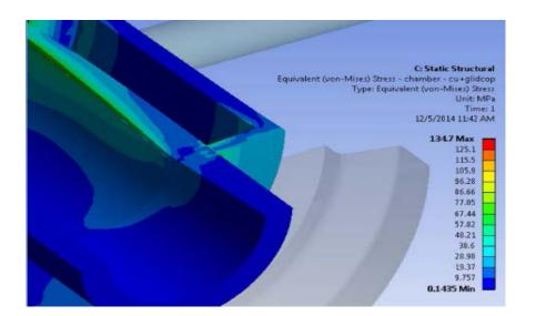
Results from ANSYS Mechanical simulation of FODO chamber end absorber thermal behavior. FODO chambers are expected to see up to 20 W/mm<sup>2</sup> on walls and 50-60 W/mm<sup>2</sup> on "in-line" absorbers needed to protect BPM/bellows and pump liners. *Courtesy B. Brajuskovic*
