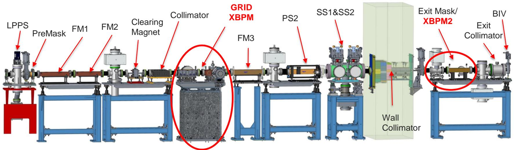
A high heat load front end layout for APS Upgrade
