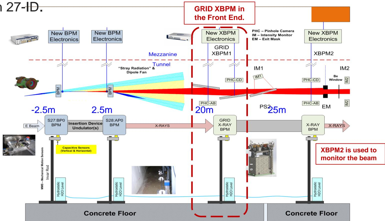
The long lever arm (along with using the x-rays) results in better capabilities for XBPM over RF-BPM
