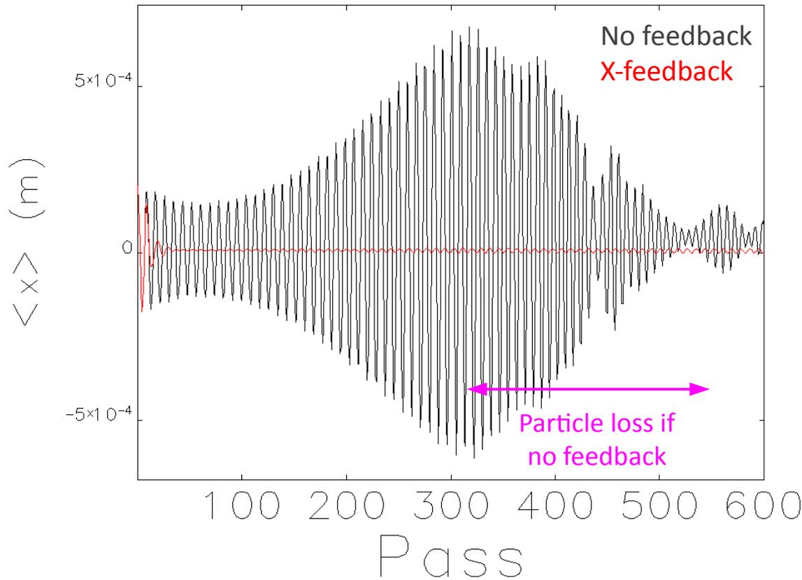
Longitudinal evolution differs due to differing amounts of particle loss
