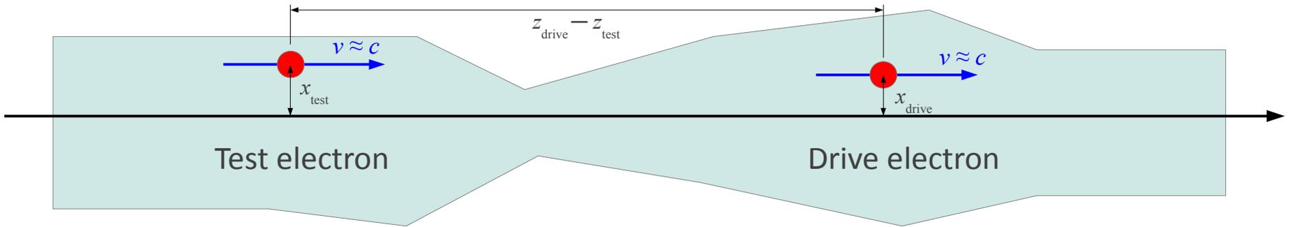
Transverse wakefields  $W_{\perp}$  change the test particle angle:  $\Delta x' = -\frac{e}{\gamma mc^2} \int_{-\infty}^{\infty} ds (\mathbf{E} + \mathbf{v} \times \mathbf{B})_{\perp} \equiv -\frac{e^2}{\gamma mc^2} \mathbf{W}_{\perp}(x, y, z)$
