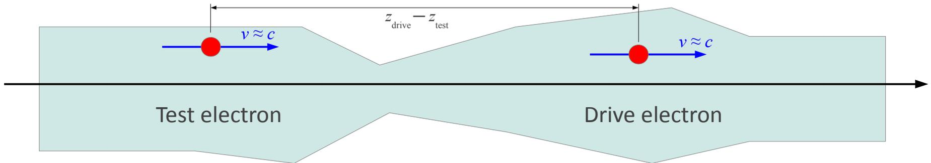
Longitudinal wakefields  $W_{\parallel}$  change the test particle energy:  $\Delta\gamma = -\frac{e}{mc^2} \int_{-\infty}^{\infty} ds E_{\parallel}(x, y, z; s) \equiv -\frac{e^2}{mc^2} W_{\parallel}(x, y, z)$
