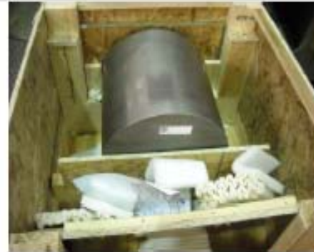
RRR>250 large grain Nb ingor
