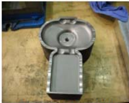
Finished first half with 4mm wall thickness
