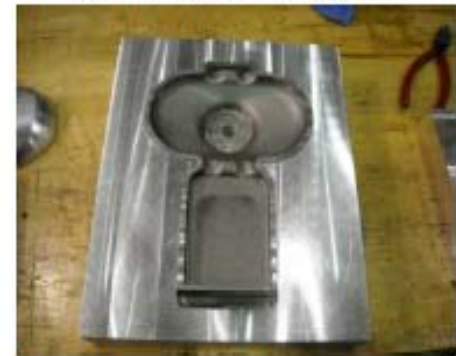
Machine inner surface on the base
