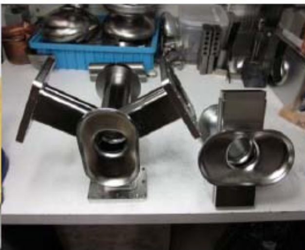
Finished two half groups before final equator EBW
