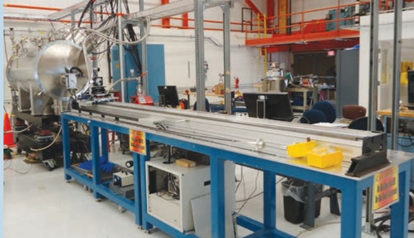
Superconducting undulator cryomodule during magnetic measurement and cryogenic testing
