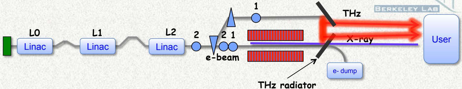
**Use two bunches in the linac and use first as THz emitter. Note that  $T_{S\text{-band}} = 330\text{-}350$  psec**
