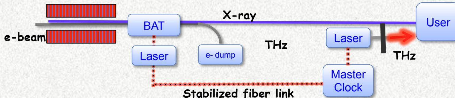
Example: Synchronized laser-based THz source
