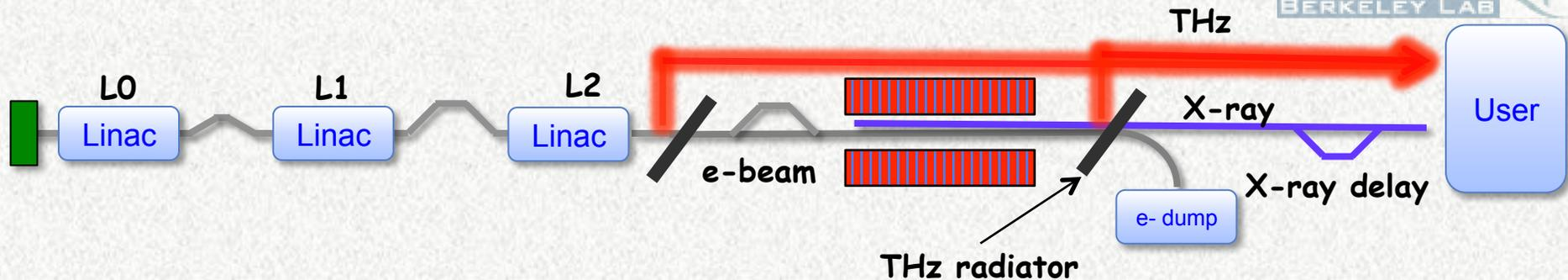
**FEL e-beam (<100 fsec, 0.1-1 nC) is natural generator of coherent THz. However, science is the driver....**
