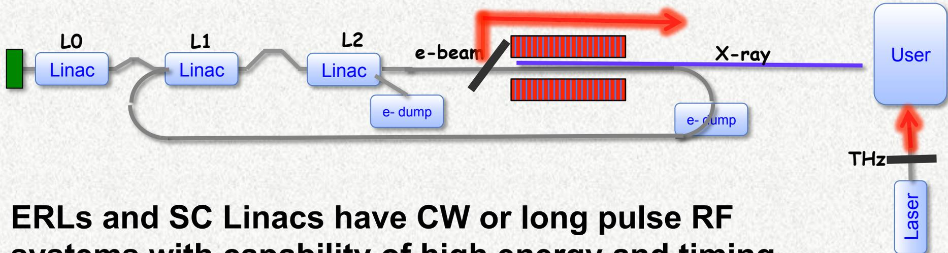
**ERLs and SC Linacs have CW or long pulse RF systems with capability of high energy and timing stability.**
