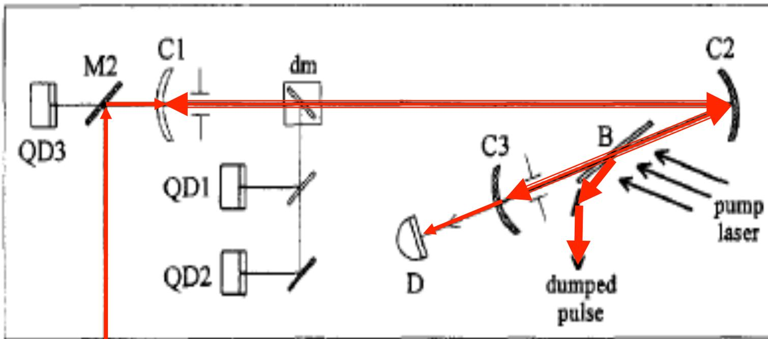
Peak power limited by cavity Q and phase stability of pulses
