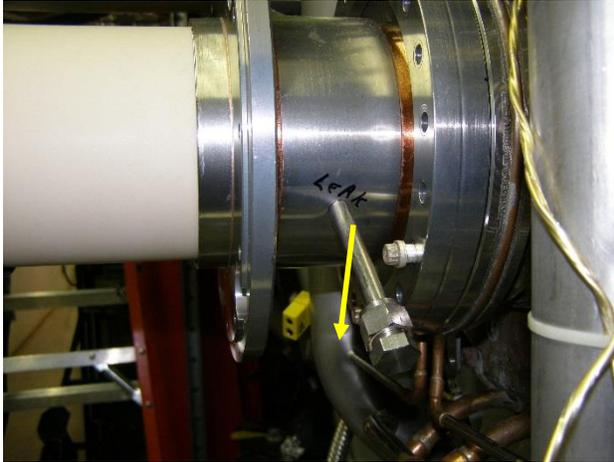
Fig. 3: Location of water leak from the unwelded body water pipe on the Sector 40/Cavity #2 input coupler.
