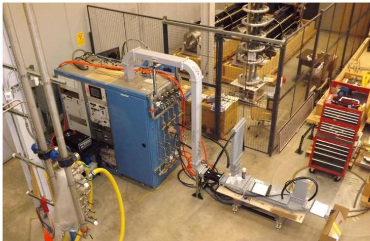
Fig. 15. Multi-Purpose Amplifier assembly in Building 400A, showing the WR-650 waveguide system and L-band isolator.
