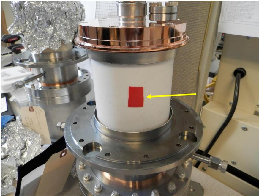
Fig. 7: Coupler ANL-28 after removal from the RF Test Stand cavity. The arrow indicates tape marking the general area of the pinhole leak.
