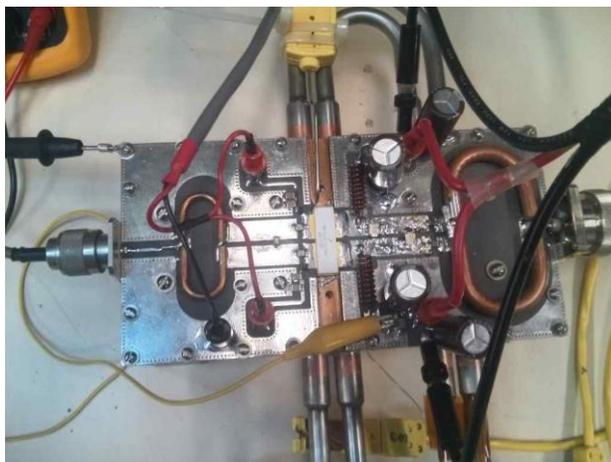
Fig. 8: Prototype 352-MHz, 2-kW amplifier on test bench
