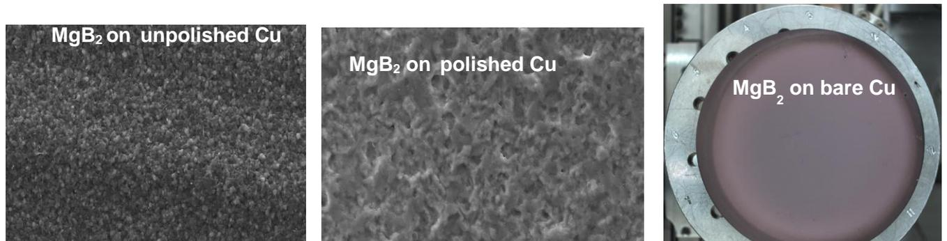
Fig. 14: SEM images of unpolished/polished bare copper coated with  $MgB_2$ . The images show of polished Cu show smaller grains compared to the large grains seen on unpolished copper. A uniform and dense  $MgB_2$  growth on bare copper is also observed.
