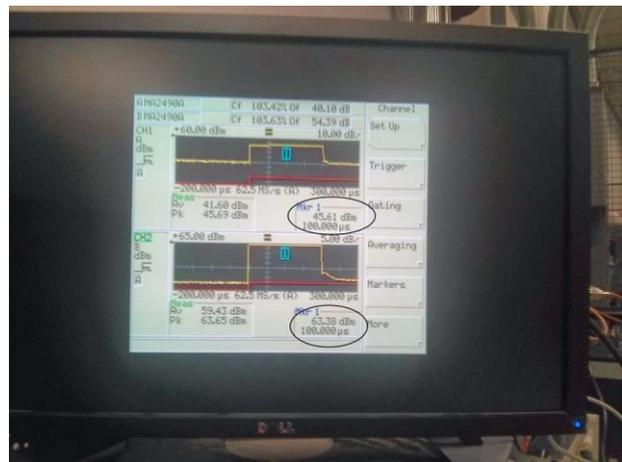
Fig. 9: RF power meter display indicating 2,177 watts peak output power.
