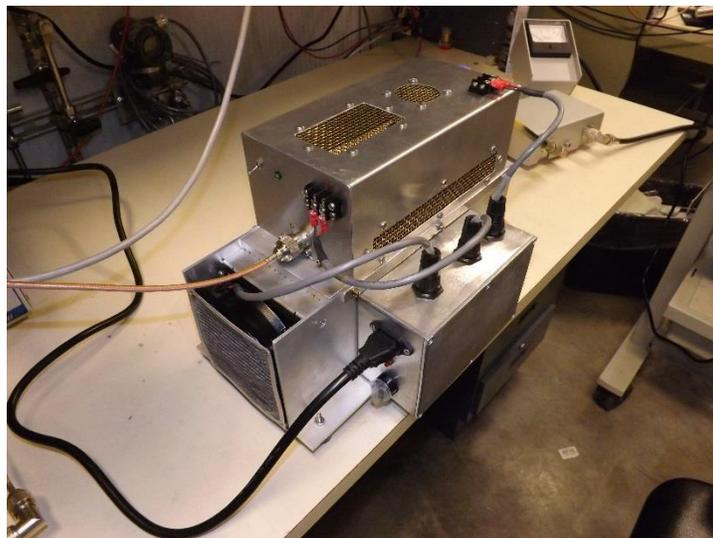
Fig. 13. 9.77MHz prototype amplifier #2 fitted with shield cover and 24-volt dc power supply box.
