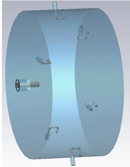
Fig. 12. Simulation rendering of the 6-input, 352-MHz/12kW cavity combiner, showing input coupling loops and output coupling post.
