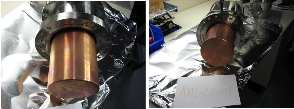
Fig. 6: New Booster tuners ANL-BT-01 and ANL-BT-02.
