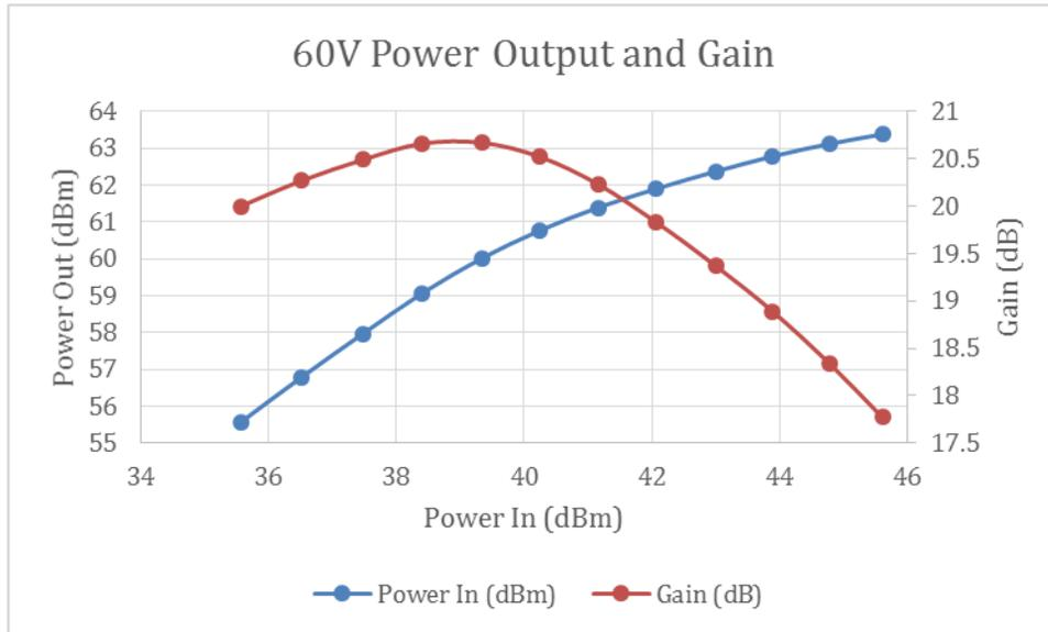
Fig. 10. RF output, input, and gain data.
