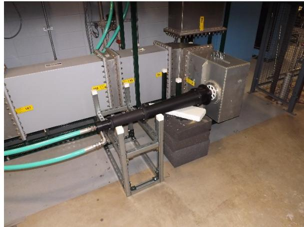
Fig. 10. The CCR load installation at the test stand, just prior to attachment to the waveguide transition.
