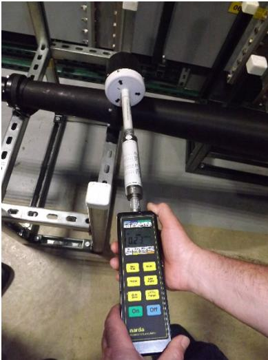
Fig. 11. RF field leak detected at second load body flange.
