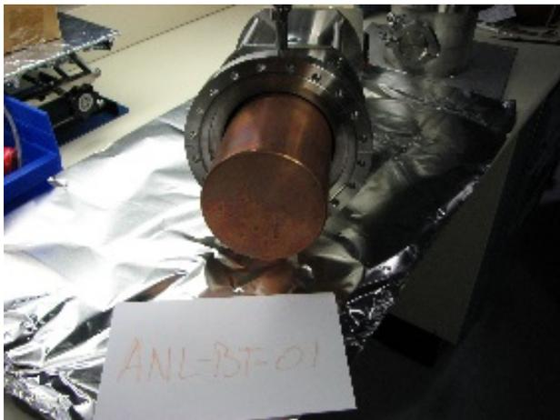
Fig. 7. Booster tuner ANL-BT-01 prior to installation in rf test stand cavity for conditioning.
