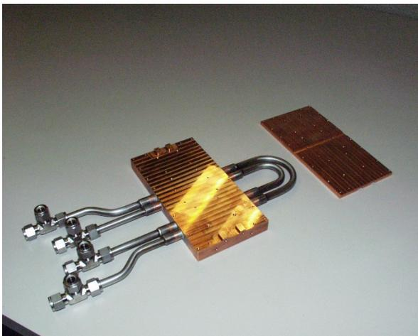
Fig. 13. The first carrier/cold-plate assembly.
