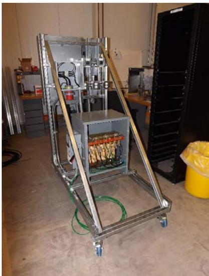
Fig. 22. MPA portable ac power distribution panel.
