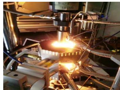
**Fig. 6.** Innovative load frame and thermal-gradient furnace that mimics the *operando* conditions in turbine engines. Knipe et al., Nat. Comm. **5**, 4559 (2014)
