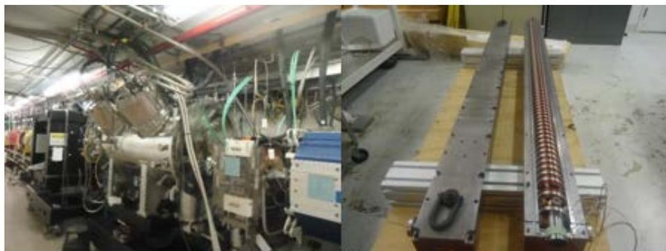
**Fig. 17.** SCU18-2 in Sector 6 of the APS ring (left); the high-temperature superconducting magnet in the impregnation mold (right).
