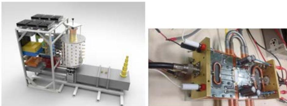
**Fig. 18.** Left shows a conceptual layout of a Solid-State rf source at 352 MHz. Individual sources at a few kW each feed a combiner cavity that couples power to a waveguide. The right image shows a single 2 kW amplifier developed in the ASD rf Group.
