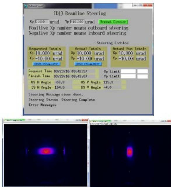
**Fig. 25:** User interface screen (top). Examples showing 10- $\mu$ rad steering outboard (bottom left) and 10- $\mu$ rad steering down (bottom right). Courtesy of Peter Eng, The University of Chicago, GeoSoilEnviroCARS-CAT.
