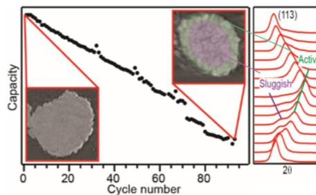
**Fig. 2.** *Operando* x-ray diffraction revealing how inter-granular cracking leads to two populations of battery grains with different reaction kinetics. Nano Lett. **17**, 6 (2017).
