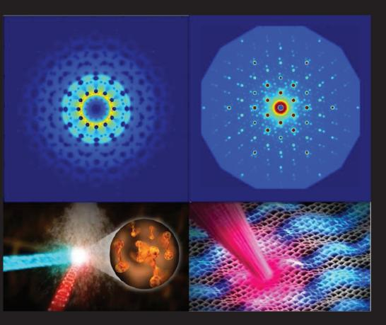
MeV-UED. The rotational wave-packet dynamics of non-adiabatically laser-aligned nitrogen molecules and atomically resolved movies of coherent nuclear motion in iodine molecules were imaged using MeV-UED. Recently, molecular movies of chemical bond breaking, ring-opening, and nuclear wave-packet passing through conical intersections were successfully recorded at SLAC MeV-UED.
