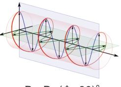
$B_{x} = B_{y} (\Phi = 90)^{\circ}$
