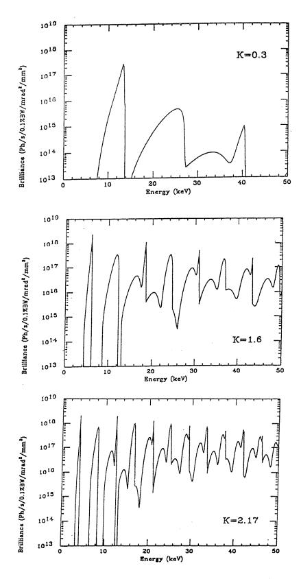
Figures 3.3.2 - 3.3.4 Energy spectra of radiation from Undulator A for three values of K. The positron beam parameters in these calculations are: horizontal beam width  $\sigma'_X$ : 308 µm, vertical beam height  $\sigma'_Y$ : 85 µm, horizontal beam divergence  $\sigma'_X$ : 24 µrad, vertical beam divergence  $\sigma'_Y$ : 9 µrad
