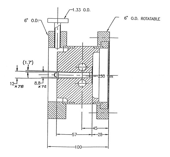
Fig. 3.5.2 Window for wiggler white beam and wiggler/undulator monochromatic beam
