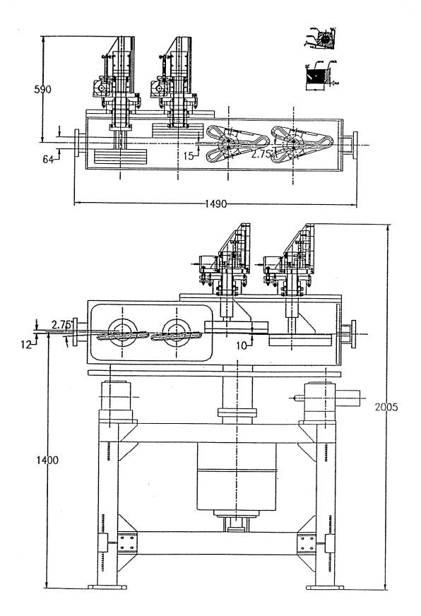
Fig. 3.5.6 ID white beam horizontal and vertical slits
