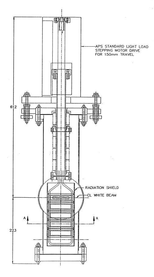
Figure 3.5.1 APS beamline filter assembly
