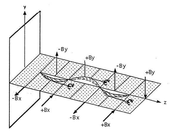
Figure 3.3.6 Placement of magnetic field components to generate circularly polarized radiation from the elliptical motion of positrons in a wiggler. The  $B_x$  and  $B_y$  components have a special phase difference of  $\pi/2$  along the z axis. In this case, the on-axis radiation is right circularly polarized (Ref. 5)
