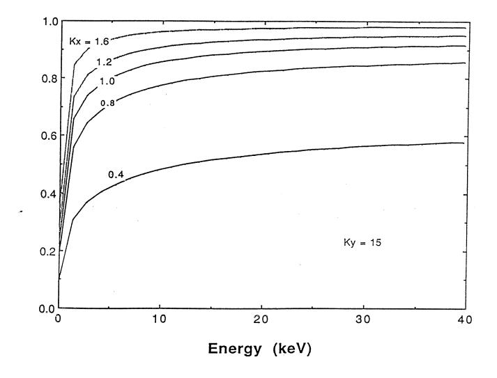
Figure 3.3.8 Variation of  $P_c$  as a function of photon energy for the elliptical motion wiggler with a period of 15 cm operated at 7 GeV for  $K_y = 15$  and various values of  $K_x$
