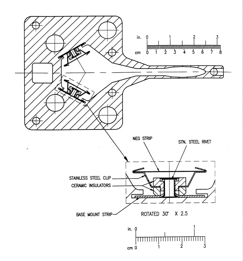
Figure 3.3.10 Cross section of the ID vacuum chamber
