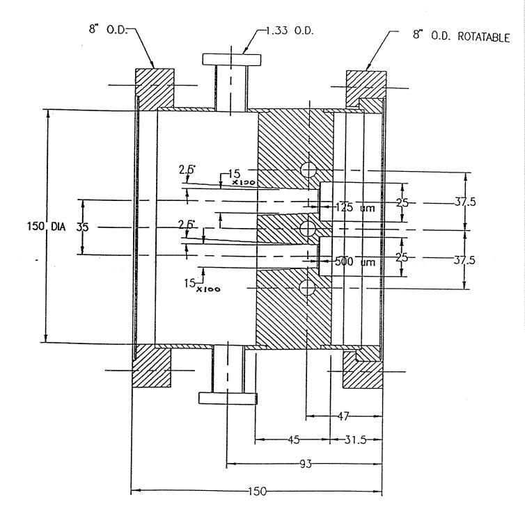
Fig. 3.5.3 Monochromatic and white beam dual window
