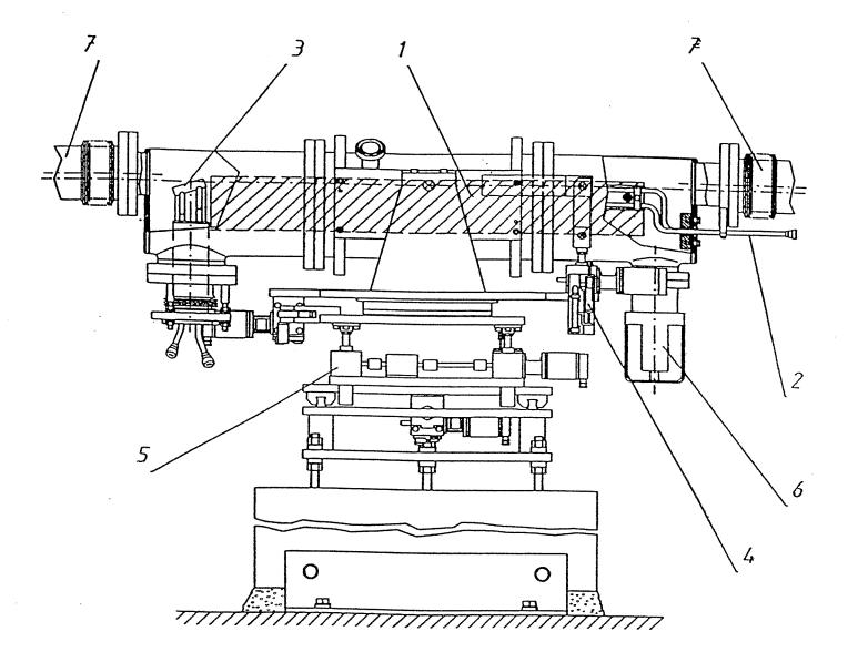
Fig. 3.5.10 X-ray mirror chamber for high power beamlines
