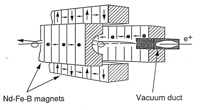
Figure 3.3.7 Conceptual design for the elliptical motion wiggler
