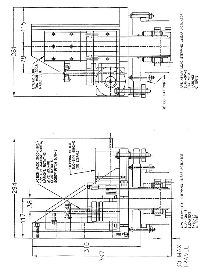
Fig. 3.5.12 APS heavy load stepping linear actuator
