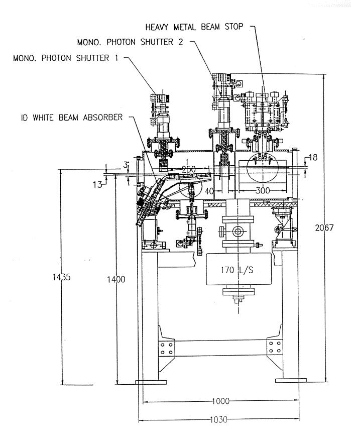
Fig. 3.5.9 White and monochromatic integral shutters and stops
