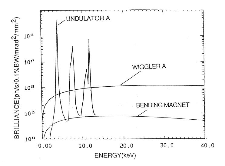
Figure 3.3.1 A comparison of the on-axis brilliance for the APS bending magnet source, Wiggler A, and Undulator A
