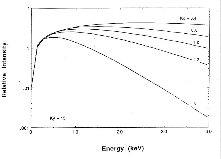
Figure 3.3.9 On-axis relative intensity of the circularly polarized beam as a function of photon energy for various values of  $K_X$
