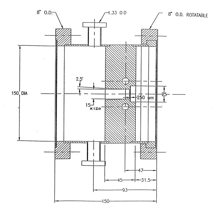
Fig. 3.5.4 Bending magnet white beam window
