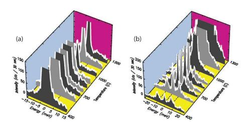
Fig. 1. Quasi-elastic scattered x-rays show a large peak in intensity at temperatures below about 880° C [middle peak in both (a) and (b)], suggesting the material is frozen in a glassy state.
