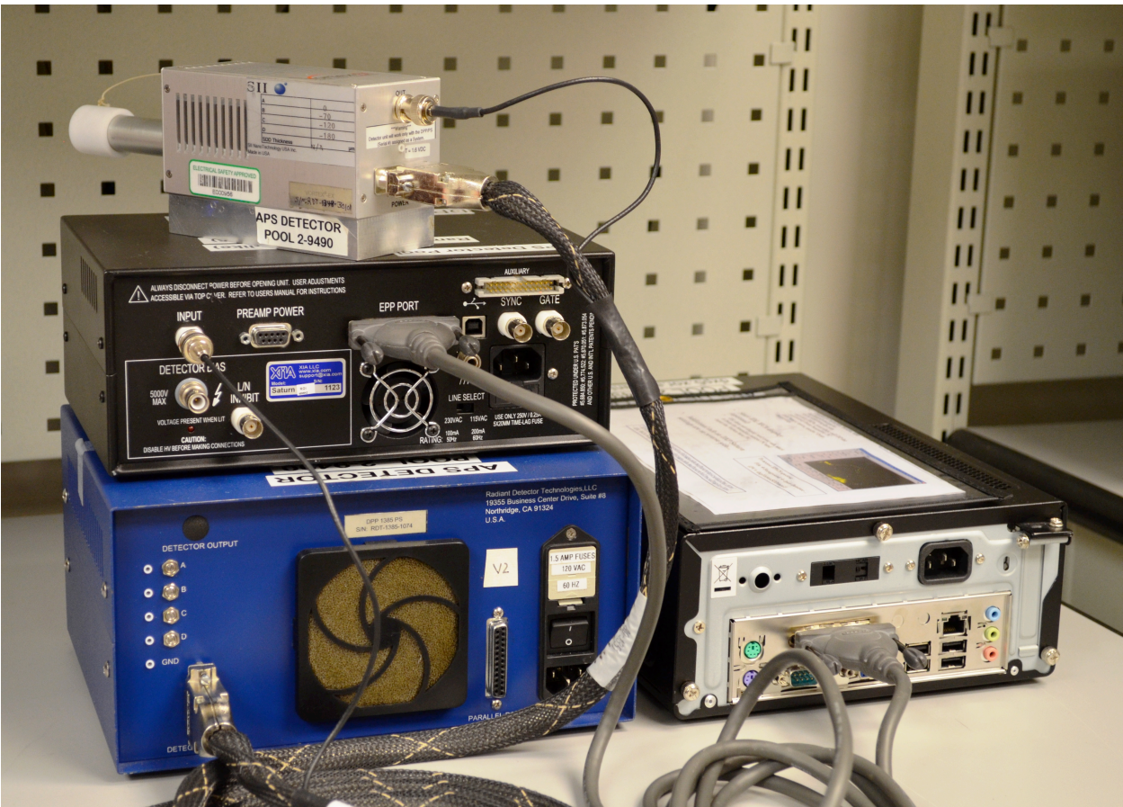
Figure 4 : Vortex detector with external DXP-Saturn unit. Note that the parallel port cable connects the computer to the Saturn box, not the blue power supply box.
