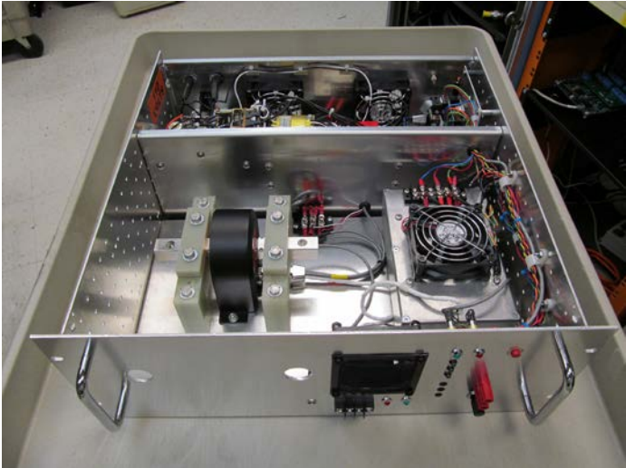
Fig. 2. DCCT chassis developed to perform precision current measurements for APS-U power supplies.
