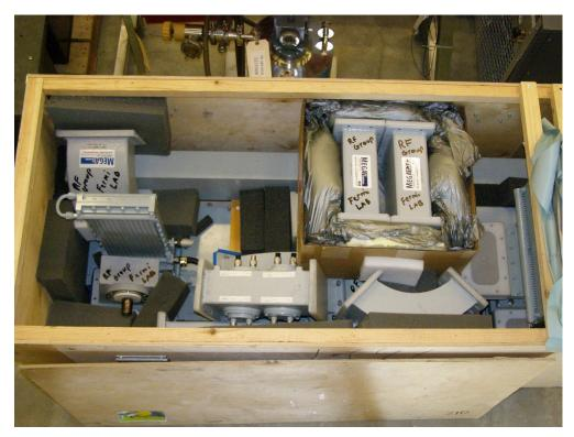
Fig. 24. WR-650 waveguide components necessary to build L-band test system for the MPA.
