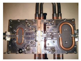
Fig. 15. The first 352-MHz/2kW prototype amplifier after electrical assembly.
