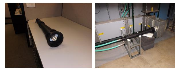
Fig. 9. The CCR 200kW rf load as received.
