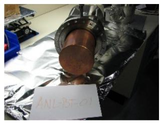
Fig. 7. Booster tuner ANL-BT-01 prior to installation in rf test stand cavity for conditioning.
