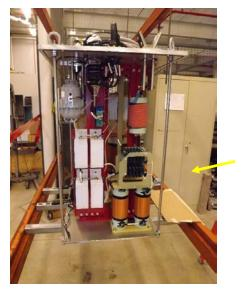
Fig. 23. Threaded rod replacement on MPA high voltage tank.
