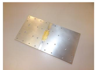
Fig. 14. The first Euclid heat spreader with blank transistor flange attached by soldering.
