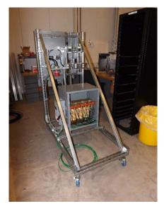
Fig. 22. MPA portable ac power distribution panel.
