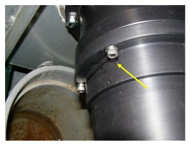
Fig. 12. Water leak from weep hole in load body.
