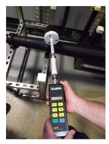
Fig. 11. RF field leak detected at second load body flange.
