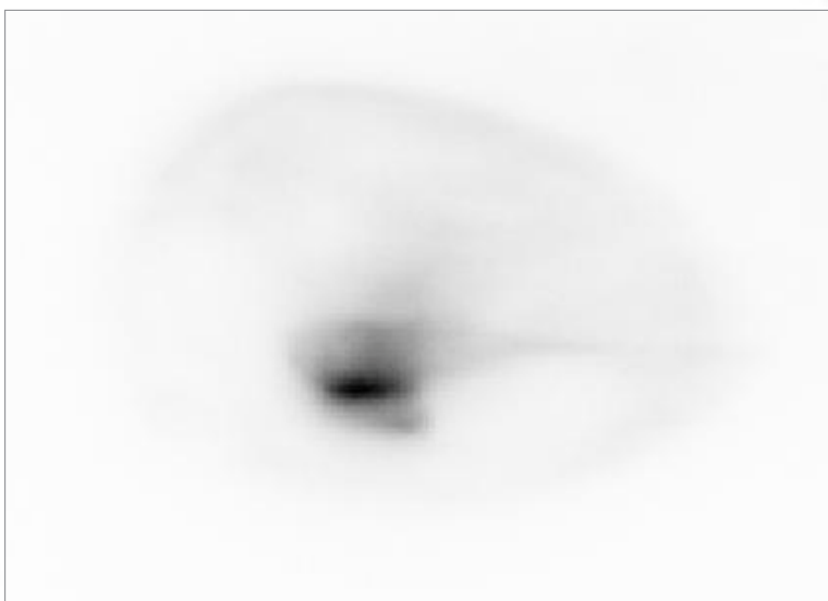
Fig. 2. A 23-fold demagnified image of the (2-sigma) 680-µm-wide and 28-µm-high x-ray source on 7-ID.
