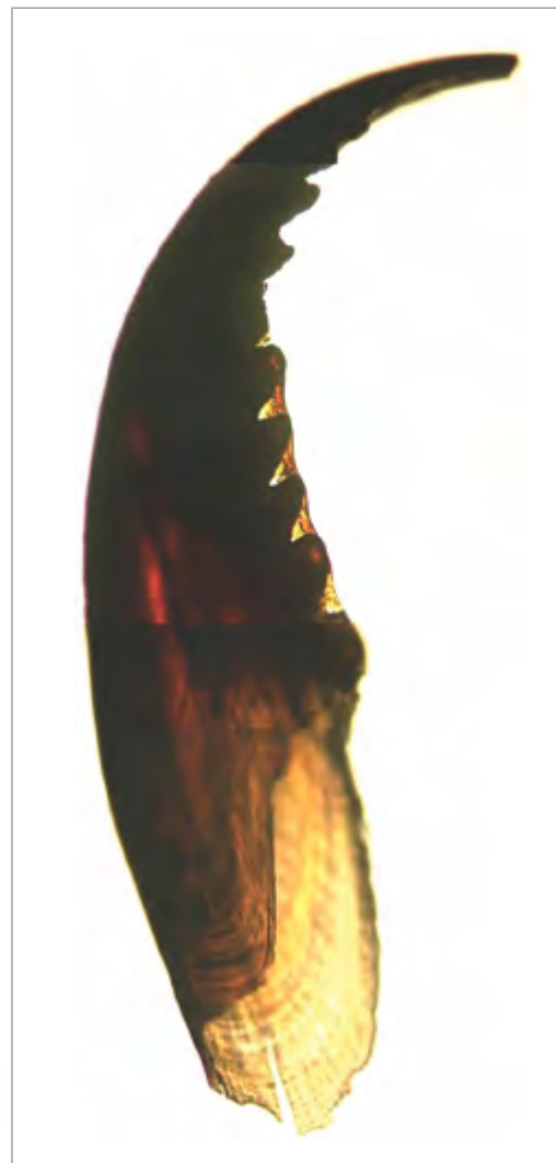
Fig. 1. The jaw of a Nereis limbata worm. The jaw is about 5 mm long, hollow at the base and solid at the tip. Higher x-ray absorption is found at the tip, indicating that that area has higher local electron density. All of the zinc is concentrated in the tip region of the jaw, with no or very low levels of zinc at the base.
