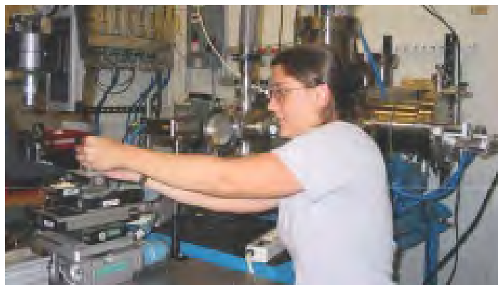
Fig. 2. Amy Grove, a senior Civil Engineering major at Cornell University, shown in the GSECARS 13-BM tomography station aligning a sediment/barrier core prior to collecting images of several sediment/reactive barrier systems. Her work is part of a pilot-scale study conducted at the University of New Hampshire and funded by the Cooperative Institute for Coastal and Estuarine Environmental Technology and the Hazardous Substance Research Center South/Southwest.
