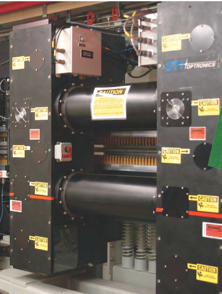
canted undulators installed at sector 23 on the APS storage ring.
