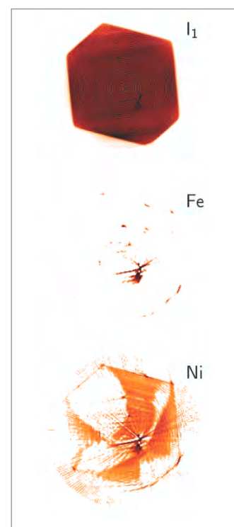
Fig. 2. Transmission and fluorescence tomograms. From the transmission data, the density of diamond (top) displays the orientation of the analyzed horizontal plane with four \{111\} faces and two \{100\} faces. Reconstructed iron and nickel fluorescence virtual slices are shown as labeled.
