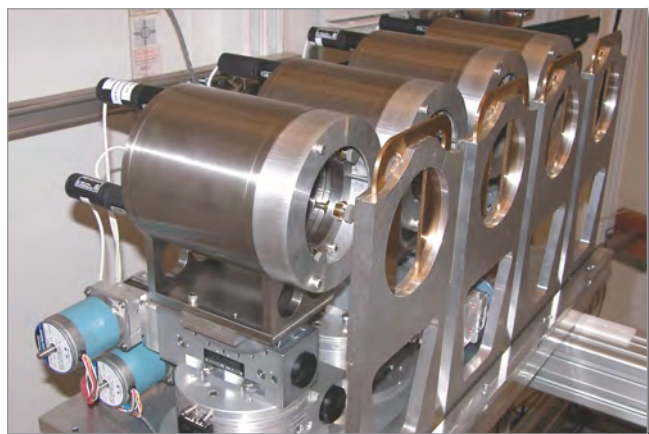
Fig. 2. Four-analyzer setup in the back of the 2-theta arm.
