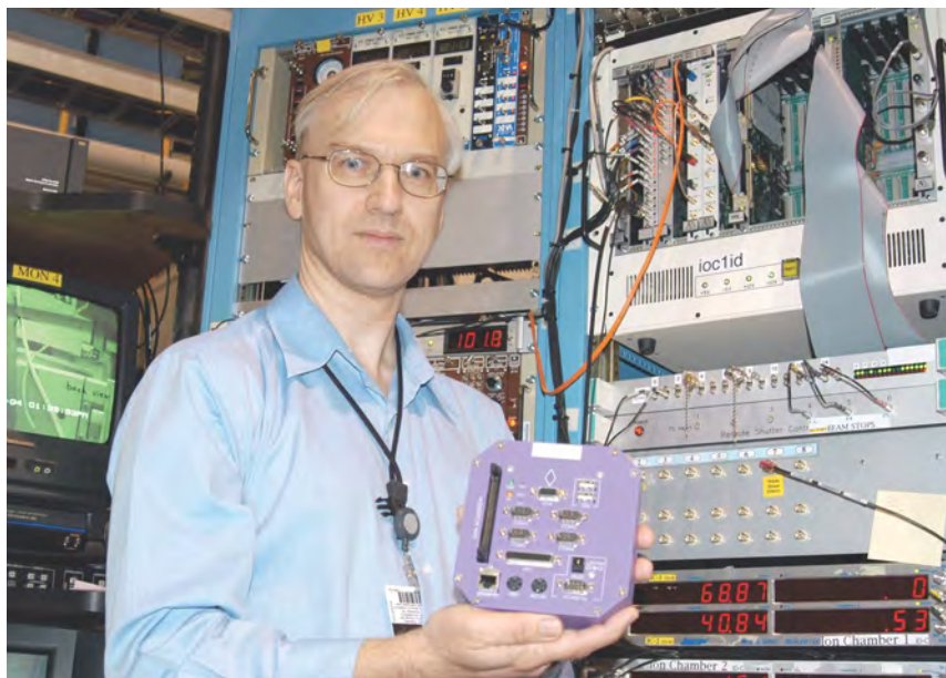
The new stand-alone EPICS IOC is shown here in the hands of Eric Norum (Controls Group), one of the developers of the device. This low-cost module, which is essentially a PC running Linux, can be used to implement an EPICS control system with much of the capability as the entire control rack seen above Eric's left shoulder.
