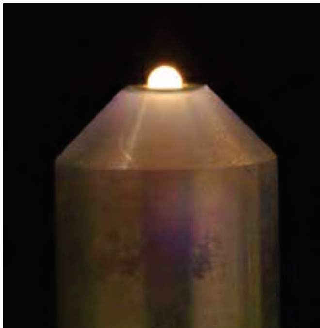
Levitated liquid-aluminum-oxide sample in a super-cooled state at \sim 1800^\circ\text{C} . The sample is levitated by an oxygen gas stream and heated by a 270-W \text{CO}_2 laser. The article reports on inelastic x-ray measurements performed on this sample.
