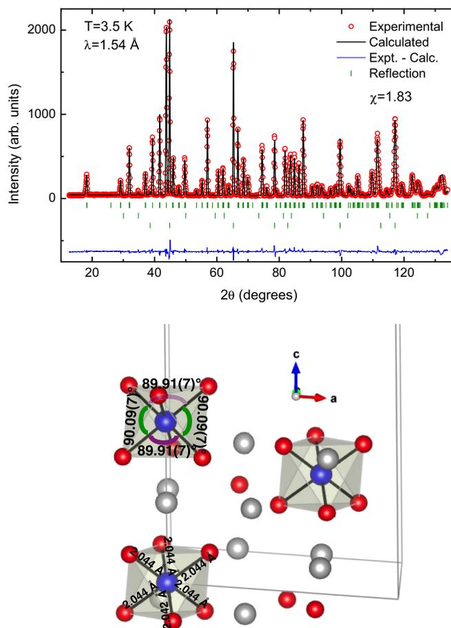
FIG. 1. (Color online) Neutron powder diffraction measurements of the crystal structure of  $\text{Sr}_4\text{RhO}_6$ . The green tick marks correspond to  $\text{Sr}_4\text{RhO}_6$ , a small impurity phase of SrO, and the Al sample can from the top down, respectively. The bond angles and distances are shown between the O (red) and Rh (blue) ions in  $\text{Sr}_4\text{RhO}_6$ , revealing near ideal and isolated octahedra. The Sr ions are shown as gray spheres.
