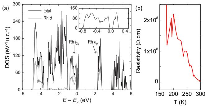
FIG. 4. (Color online) (a) DFT calculations show the  $\Gamma_1$  magnetic ordering is the lowest energy and insulating in  $\text{Sr}_4\text{RhO}_6$ . The region around the Fermi energy is shown in the inset. (b) The insulating nature was experimentally probed with resistivity measurements. The resistance increased with decreasing temperature, becoming immeasurably high below 160 K.
