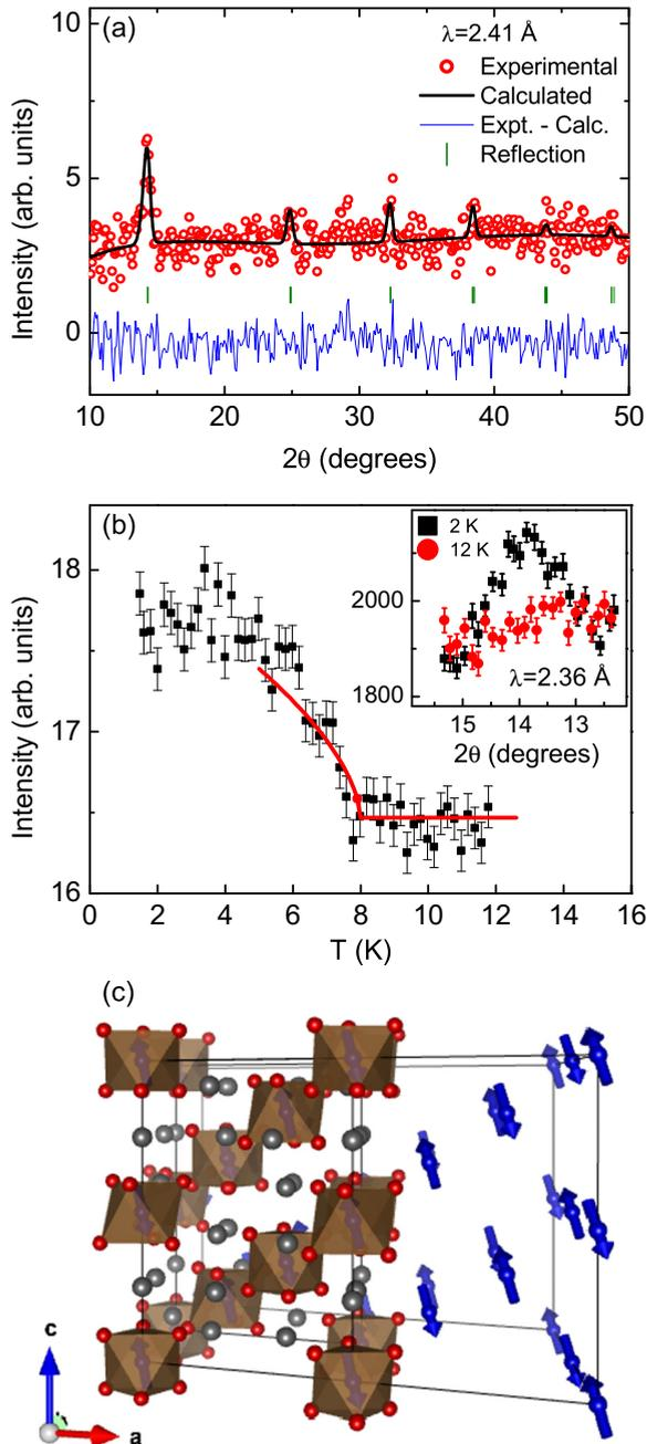
FIG. 2. (Color online) (a) Difference of 15 and 3 K neutron powder diffraction measurements. The fit is to the  $\Gamma_1$  IR magnetic model. (b) The intensity of a magnetic reflection reveals long range magnetic ordering at 7.4(5) K in  $\text{Sr}_4\text{RhO}_6$ ; the fit is to a power law. (c) The lowest energy  $\Gamma_1$  magnetic ordering in  $\text{Sr}_4\text{RhO}_6$ .
