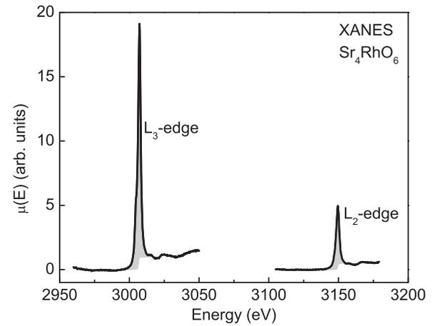
FIG. 3. Normalized and self-absorption corrected XANES fluorescence measurements through the  $L_2$  and  $L_3$  edges in  $\text{Sr}_4\text{RhO}_6$ . The peak in the white line occurs at  $L_2 = 3149.0 \text{ eV}$  and  $L_3 = 3007.12 \text{ eV}$ . Measurements were performed at room temperature.
