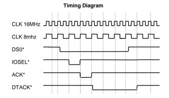
A Time-out error will result for the following condition if Auto Acknowledge is disabled in the carrier status register.
