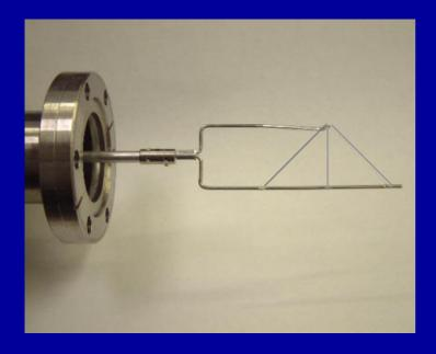
A typical wire scanner (WS) at Jefferson Lab
