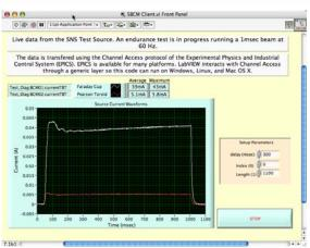
Channel Access Client interface for LabVIEW to serve as data client for console applications
