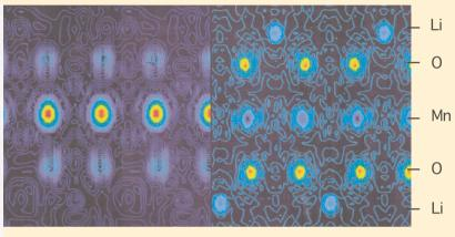
Material for Li-battery seen by X rays (left) and
