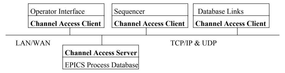
Client: Provides read/write connections to any subsystem on the network with a channel access server
