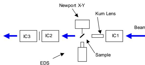
FIG. 1. Schematic representation of the instrumental arrangement. IC = ion chamber, EDS = solid-state detector, Kum Lens = polycapillary optic lens.
