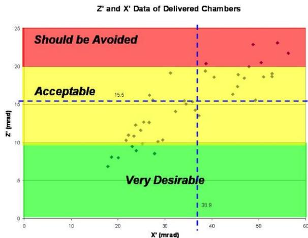
Figure 8: Graphical display of surface finish data from 46 chambers. The average of all vacuum chambers is 14.86 mrad in  $Z'$  and 35.14 mrad in  $X'$ . The rms of  $Z'$  is 15.5 mrad and  $X'$  is 36.9 mrad. Selecting the best 33 chambers yields an rms of 13.9 mrad for  $Z'$  and 34.2 mrad for  $X'$ . Five chambers were sacrificed to verify the surface finish in the middle of the extrusions.
